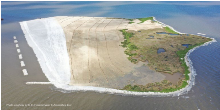
Figure 3: Example of a system-based coastal resilience strategy integrating shoreline stabilization, sediment placement, and habitat restoration. The Queen Bess Island project illustrates how adaptable design concepts can rebuild landform integrity and ecological function under dynamic coastal conditions.
