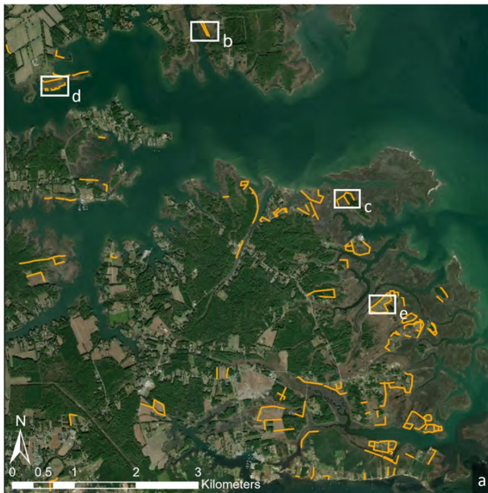
Figure 2: Map of historical berms in the Guinea marshes study area from Hall et al., 2022. Mapped levees are indicated with orange lines, and each field site is indicated with a white box, b-e. In this proposal, we would survey the elevation of the berms with RTK GPS, identify natural breaches, and determine the efficacy of berm breaches on marsh health as a design alternative for creating and restoring tidal wetlands.
