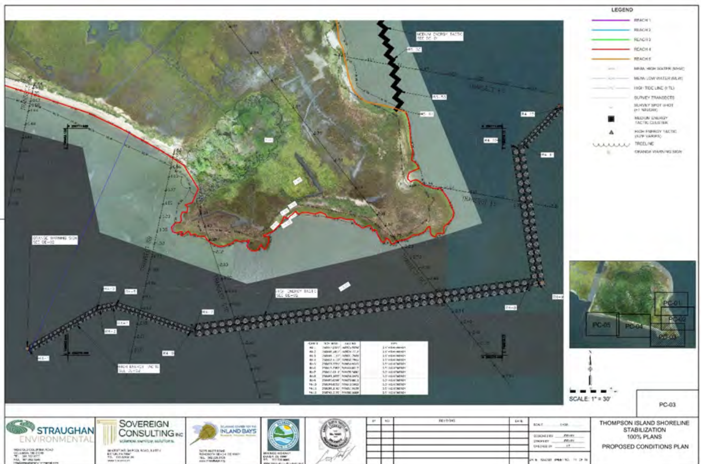
Photo 2 | Wave Attenuation Structures (WASs) are designed offshore of Thompson Island, DE to address high wave energy conditions and to protect adjacent nature base shoreline project elements.
