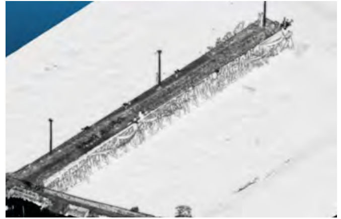
Combined 3D acoustical imaging, LiDAR, and bathymetry data at pier
