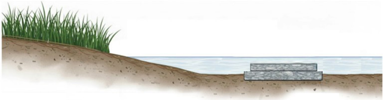
Sketch 2: Shoreline Cross-Section for a Low Wave Energy Environment
