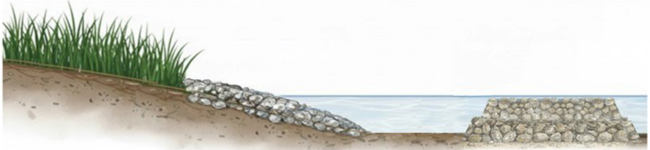
Sketch 1: Shoreline Cross-Section for a High Wave Energy Environment
