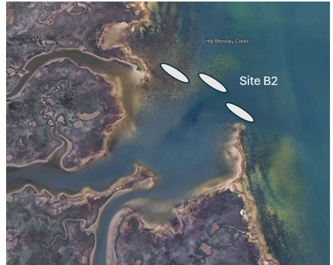
Figure 12: Conceptual arrangement of wave breaks designed to reduce wave energy within Little Monday Creek. Gaps in the wave breaks would allow navigation to pass freely.
